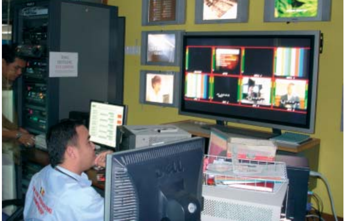
Right: The ingest area where satellite and local feeds are brought into the Quantel sQ system via Omnibus automation.
