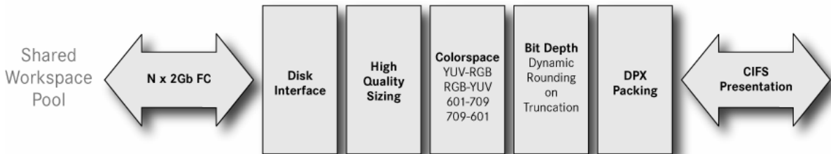
Purpose-built hardware enables on-the-fly media virtualisation
